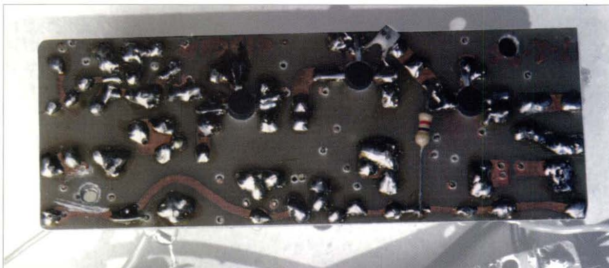
Fig. 4: As space is tight a few components must be mounted on the track side of the transmitter p.c.b.
