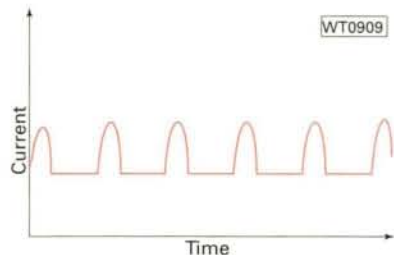
Fig. 2: The current consumption of a Gunn diode showing the current pulses.
